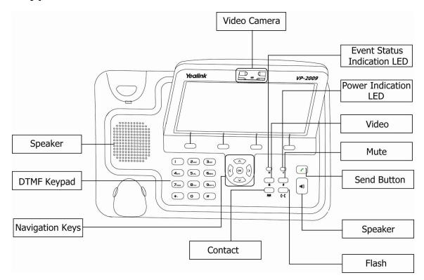
You can check the following list which introduces the IP phone's keypad in detail:
