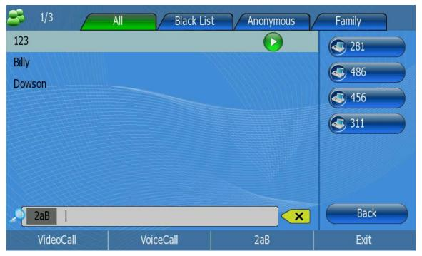
2) The registered accounts will be shown on the right side, clicking the corresponding one to dial out the chosen contact directly by this account.
